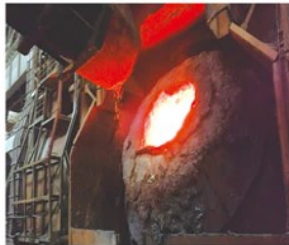
传统大面料烧结20min后依然冒出有毒烟气 Traditional material repairing: still exhaust poisonous smoke after 20min sintering.
