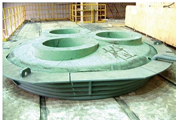
电炉小炉盖预制件 Electric furnace cover prefabs
